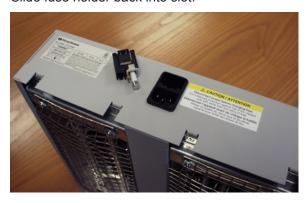
Plug in the Dryer AC power cord back into the Stacker and turn the power on. If the blown fuse condition occurs again, call Pitney Bowes for service.
